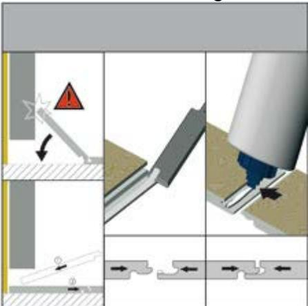
4. To start the second row, use the remainder of the last plank of the first row if it is longer than 30cm (12") long, otherwise, cut a new plank in half and proceed. To ensure structural integrity of your floor, it is mandatory to **ALWAYS STAGGER THE END JOINTS FROM ROW TO ROW BY AT LEAST 40cm (16")**.
